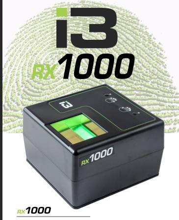
The RX1000 is usable as a free-standing device, mounted within a kiosk. or secured to a surface.
